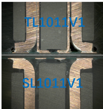
Figure 6: Convenient co-lay between TLVR inductor solutions (TL series) and single-turn standard inductor solution (SL series)
